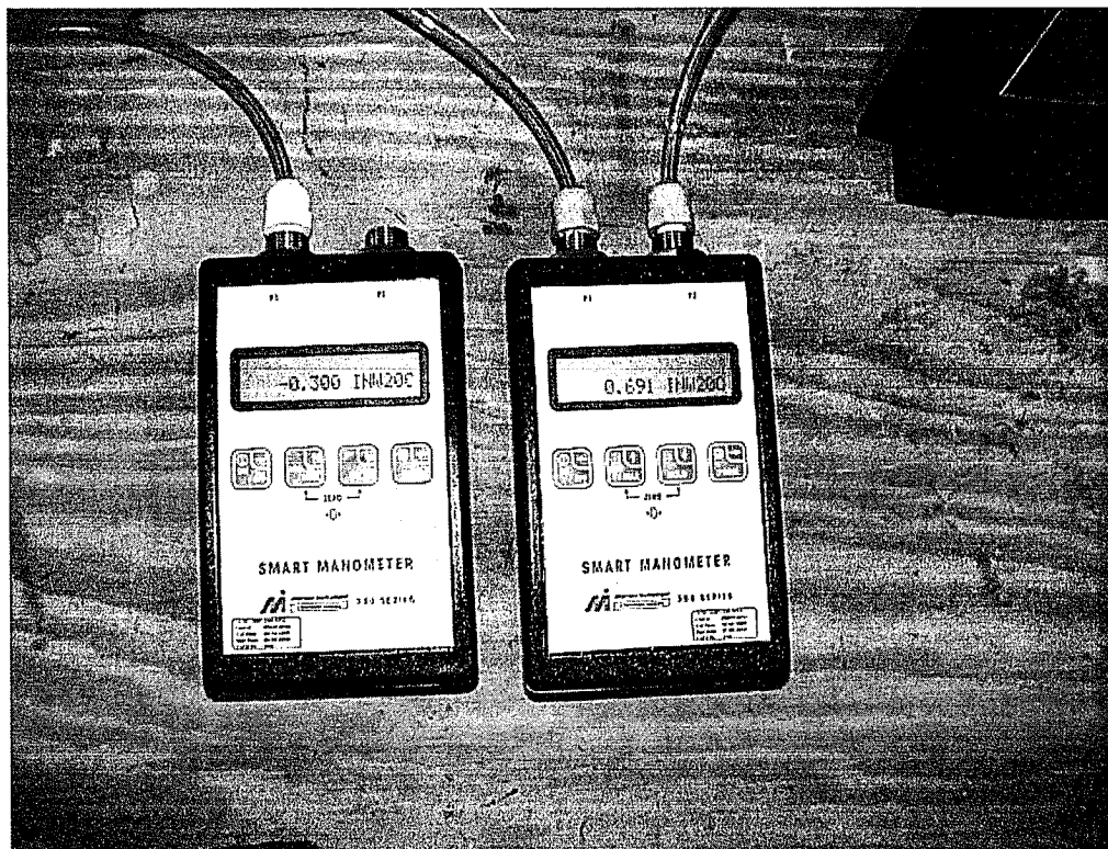
PHOTO 5 View of flow measurements at differential pressure of 1.57 psf (equivalent to 0.3" of water). (DSC00083)
