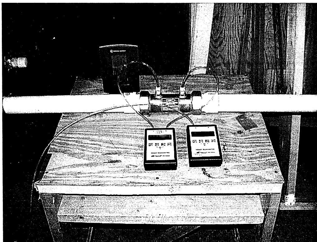
PHOTO 4 View of the air flow measuring instruments. (DSC00079)
