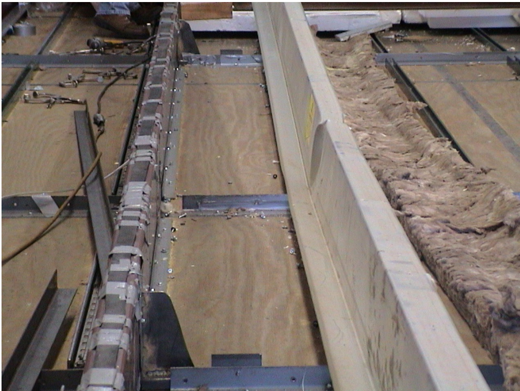
PHOTO 16 View of the flange buckling failure of 14 ga. 8" deep Zee purlin (Test #9). (DSC00141)
