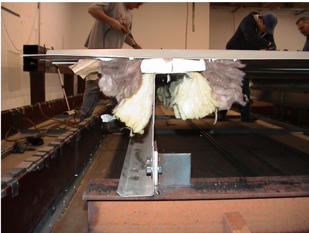
PHOTO 1 View of the purlin-frame attachment for Test #1, 2, 3, 8 & 9. (DSC00001)
