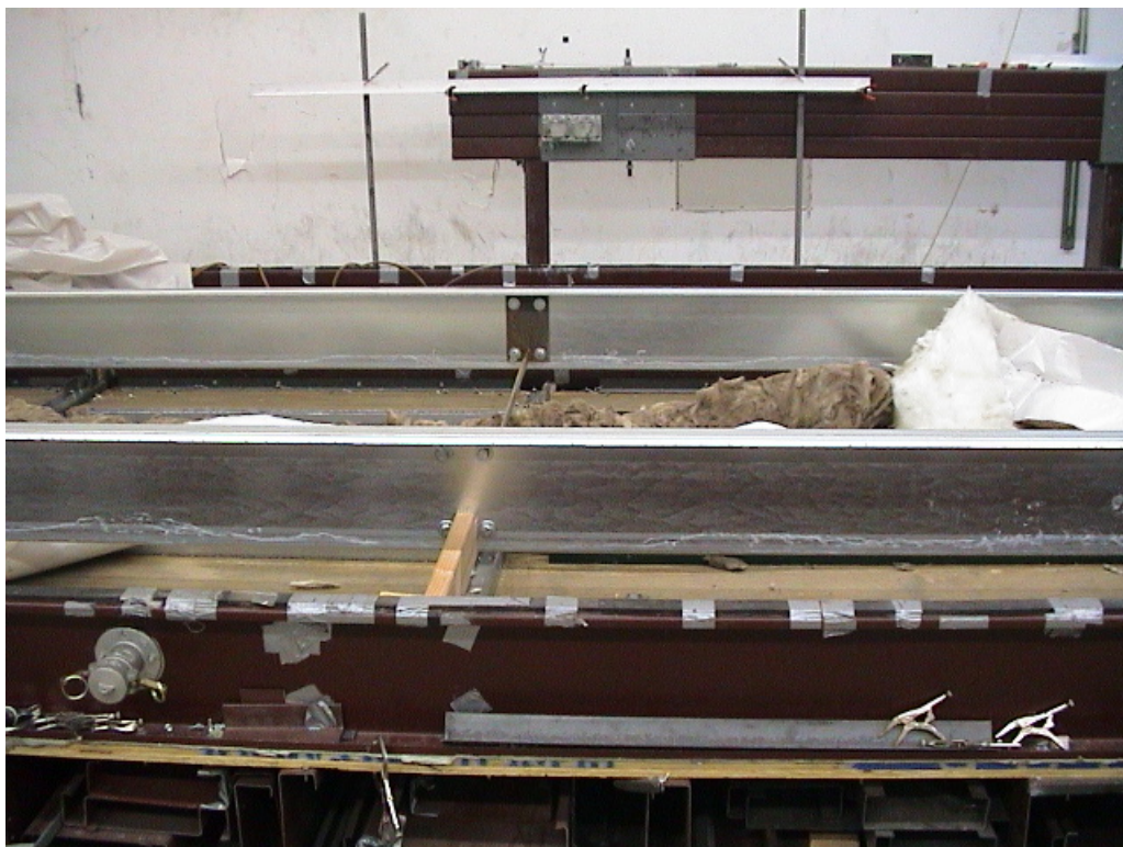
PHOTO 9 View of attachment of bracing option 3 at midspan. (DSC00146)
