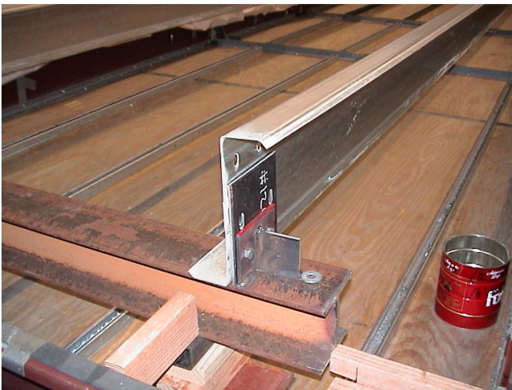
PHOTO 8 View of the purlin-frame attachment for Test #4, 5, 6, 7, 10 & 11. (DSC00102)
