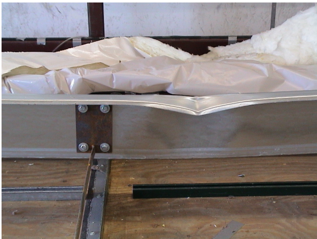
PHOTO 10 View of the flange buckling failure of 12 ga. 10" deep Zee purlin (Test #4). (DSC00112)
