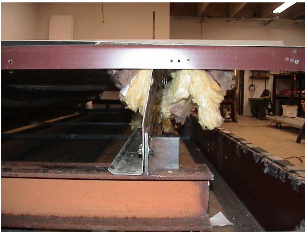
PHOTO 6 View of the web bending failure of 12 ga. 10" deep Zee purlin (Test #2). (DSC00091)
