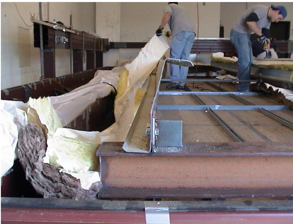
PHOTO 5 View of the web bending failure of 12 ga. 10" deep Zee purlin (Test #1). (DSC00081)
