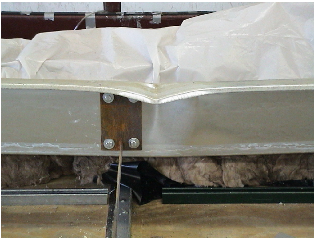
PHOTO 12 View of the flange buckling failure of 12 ga. 10" deep Zee purlin (Test #6). (DSC00037)
