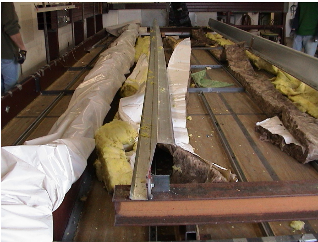
PHOTO 7 View of the web bending failure of 12 ga. 10" deep Zee purlin (Test #3). (DSC00091)
