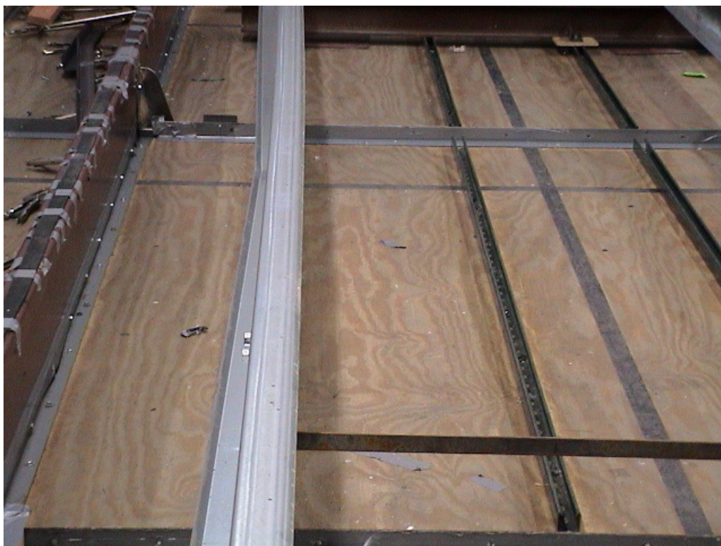
PHOTO 22 View of the bottom lip buckling failure of 12 ga. 10" deep Zee purlin (Test #12). (DSC00038)
