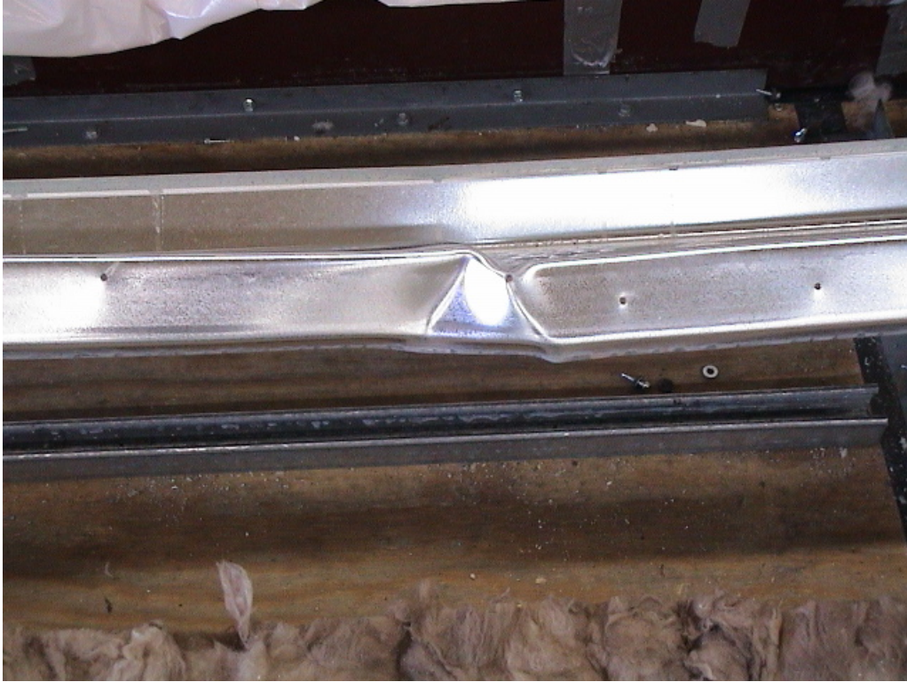
PHOTO 15 View of the flange buckling failure of 14 ga. 8" deep Zee purlin (Test #8). (DSC00137)
