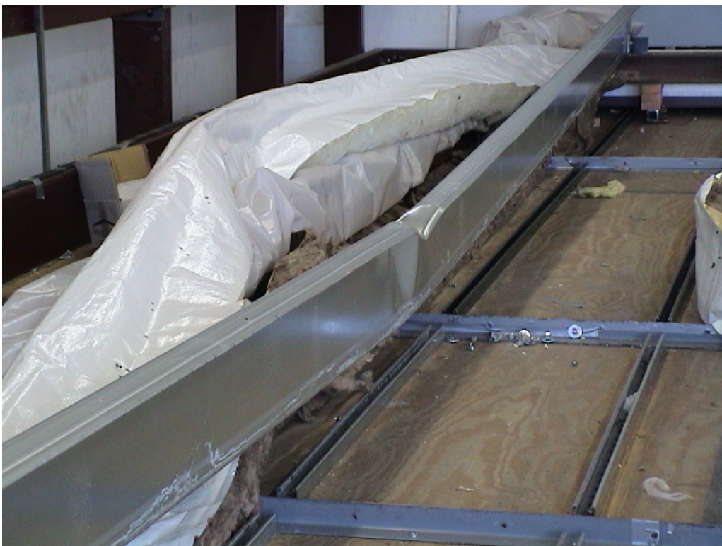
PHOTO 11 View of the flange buckling failure of 12 ga. 10" deep Zee purlin (Test #5). (DSC00034)
