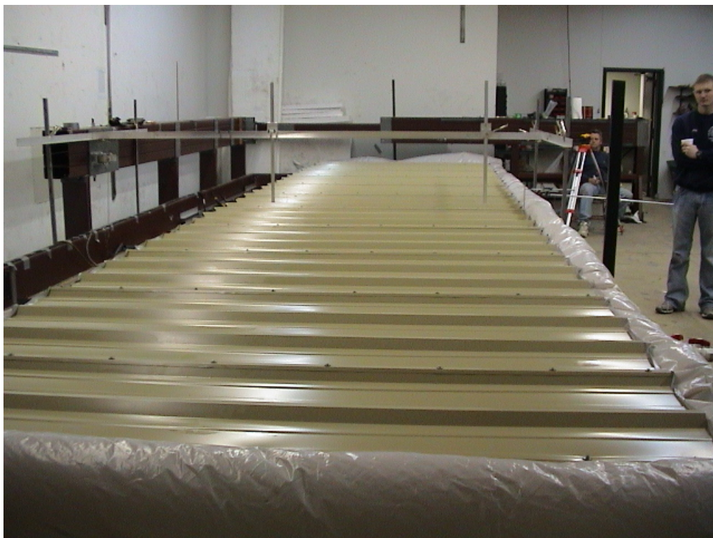
PHOTO 17 View of Test #10 under uplift load. (DSC00150)
