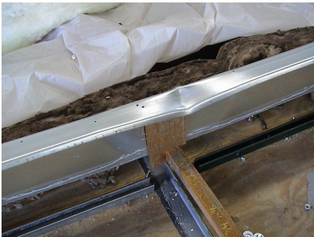
PHOTO 14 View of the flange buckling failure of 12 ga. 10" deep Zee purlin (Test #7). (DSC00132)
