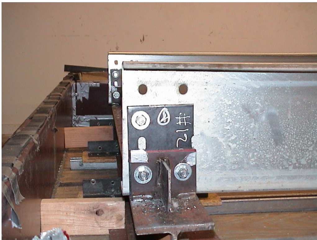
PHOTO 21 View of the purlin-frame attachment for Test #12. (DSC00036)
