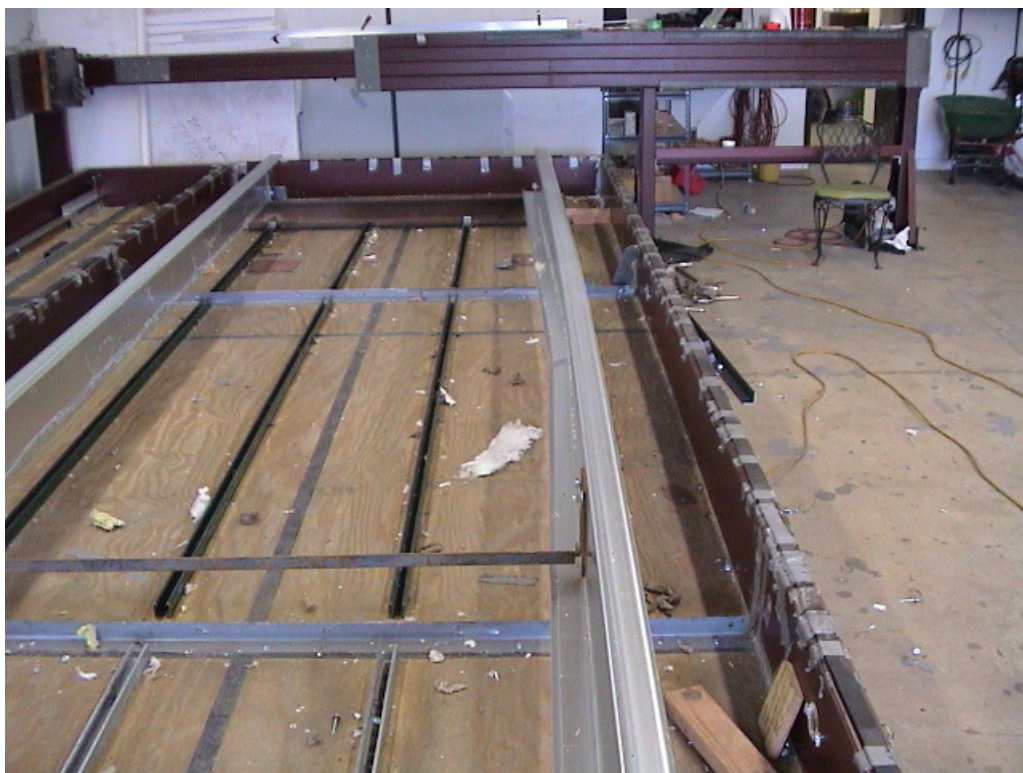
PHOTO 18 View of the bottom lip buckling failure of 12 ga. 10" deep Zee purlin (Test #10). (DSC00152)
