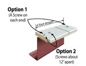
Each thermal spacer comes in six-foot lengths which are the standard widths of three Standing Seam Roof panels and the typical widths of a metal building insulation roll, making the thermal spacer easy to handle and install.
