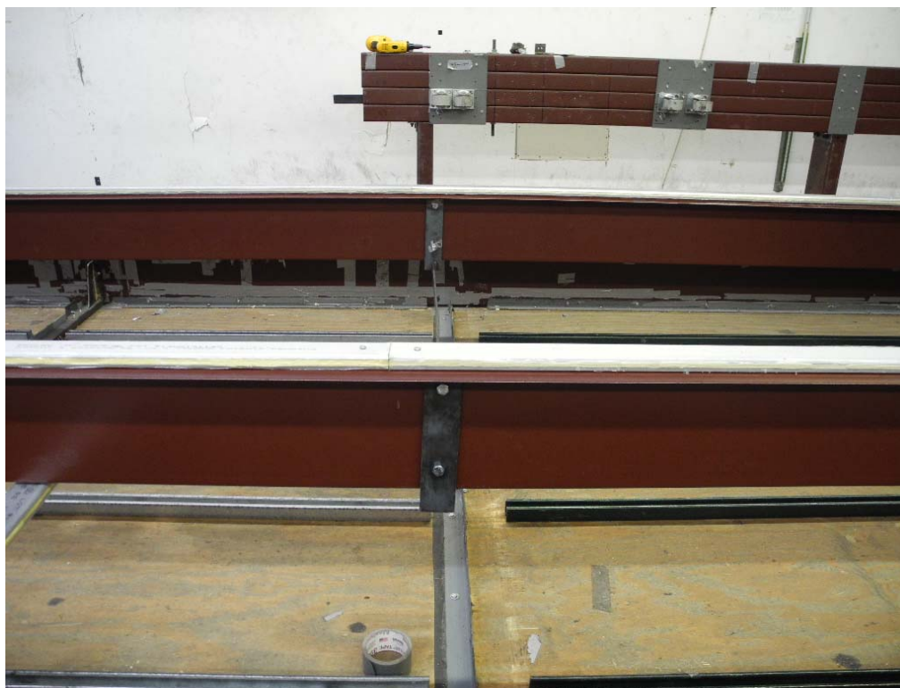
PHOTO 2 View of attachment of bracing option 4 at midspan (Test #1). (DSCN1375)
