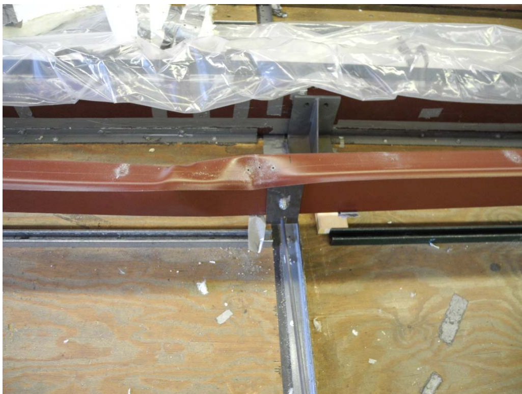
PHOTO 8 View of the flange buckling failure of 12 ga. 10" deep Zee purlin (Test #2). (DSCN1398)
