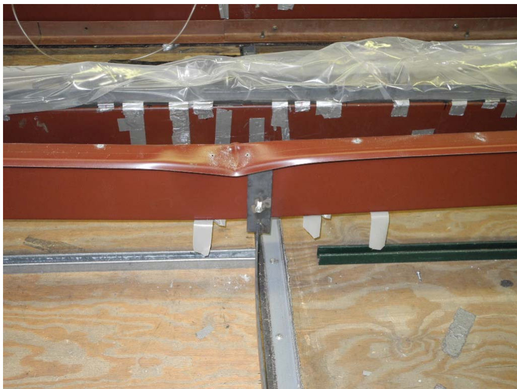
PHOTO 6 View of the flange buckling failure of 12 ga. 10" deep Zee purlin (Test #1). (DSCN1387)
