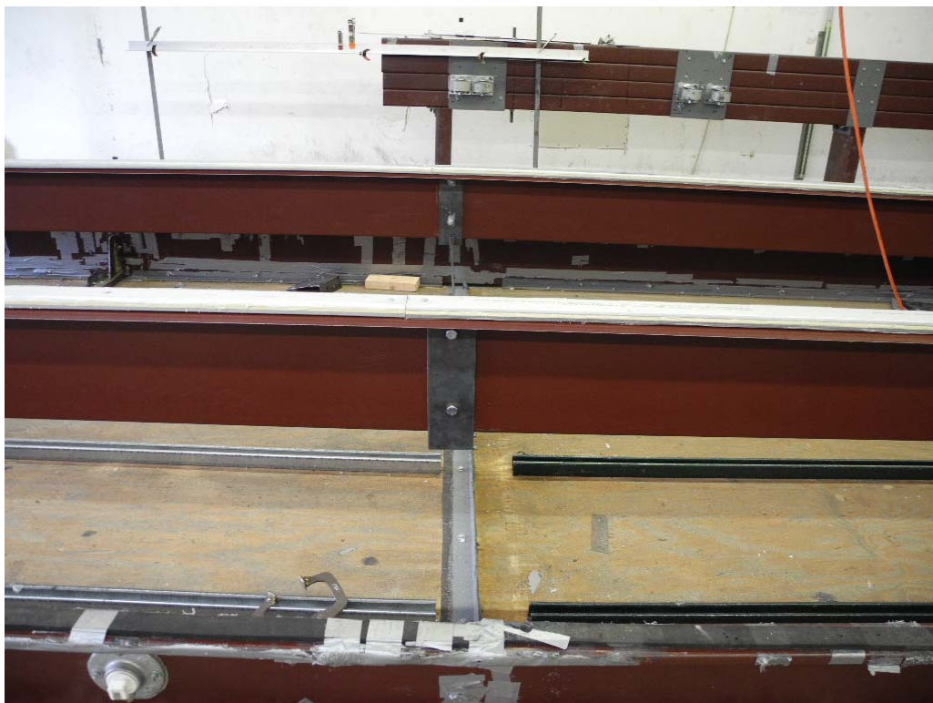
PHOTO 7 View of attachment of bracing option 5 at midspan (Test #2). (DSCN1394)
