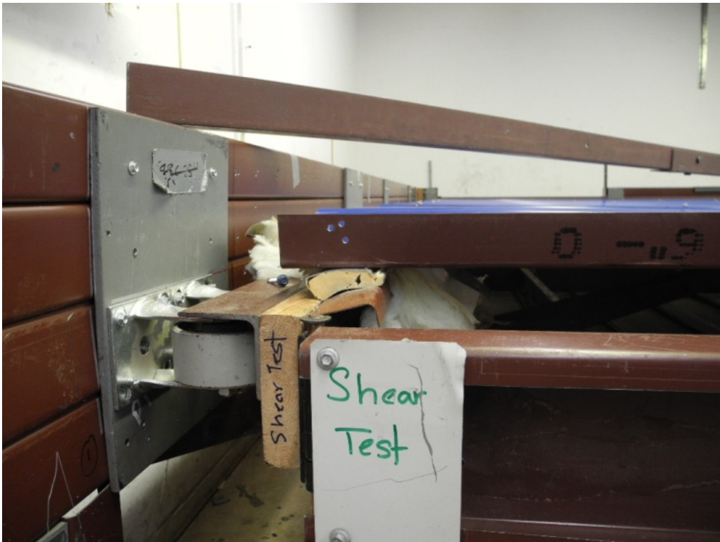
PHOTO 6 View of fastener shear failure near the roller corner in Test #2. (DSCN1373)
