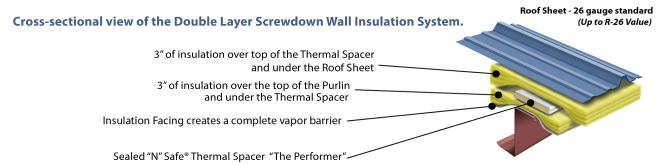
**Double Layer Roof & Wall Insulation System** (Patents Pending)
