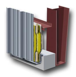
For Step 1 and 2 of the double layer system, refer to the single layer system, on the other side of this page, and do steps 1 and 2. (When installing the Insulation Blankets, offset the upper and lower insulation side joints from each other to increase efficiency)
