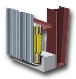
For Step 1 and 2 of the double layer system, refer to the single layer system, on the other side of this page, and do steps 1 and 2. (When installing the Insulation Blankets, offset the upper and lower insulation side joints from each other to increase efficiency)
